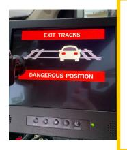
The RCVW system provides drivers with information about potential conflicts at railroad grade crossings. Drivers can be warned about activated crossing warnings using displays and audio signals in the vehicle.
