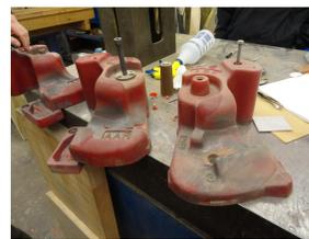
Right: Example of knuckle mold pattern used by Amsted Rail
